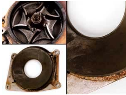
Figure 1. Original Water Pump from Caterpillar Engine with More Than 750,000 Miles Using Extended-Life Coolant (ELC).
